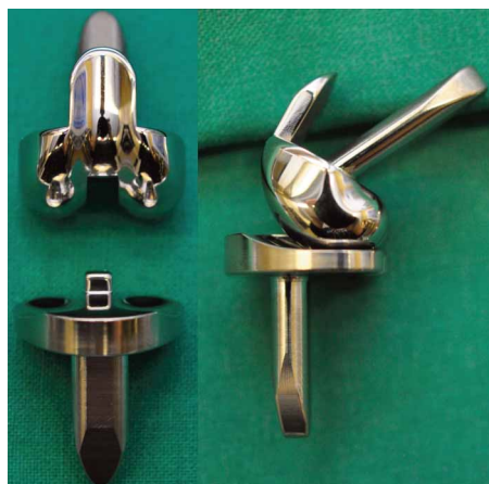
Fig. 1 Final rabbit knee prosthesis (CoCrMo), in anteroposterior (left) and mediolateral view (right)
