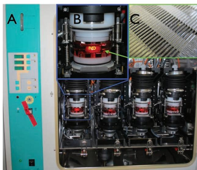
Fig. 1 Detailed view of the loading bioreactor and specimen chamber. A) The bioreactor is situated inside a 37°C incubator with 5% CO<sub>2</sub> and 80% humidity. B) The glass walled sample chamber. IVD: intervertebral disc. C) Enlarged view of the titanium plate for holding the samples for rotation movement
