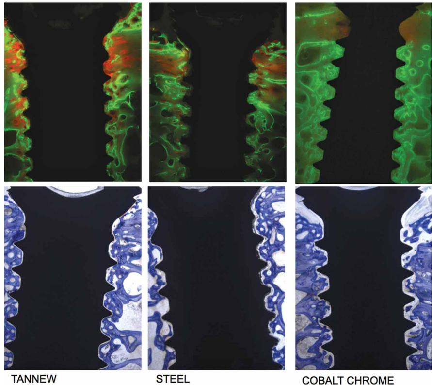
**Intravital fluorescence staining shows calcium deposition at four (green) and eight (orange) weeks. TANNEW shows significantly better osseointegration and bone remodelling compared to the standard controls, steel and cobalt chrome**
